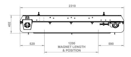
**HYD MOTOR** 1400 FRAME 1000 **HYDRAULIC MOTOR** FLOW RATE: APPROX. 40LPM (1.4M/S LINEAR **MAGNET BELT SPEED) WIDTH** 500 PRESSURE DROP: MAX 23 BAR. **BELT** 750
